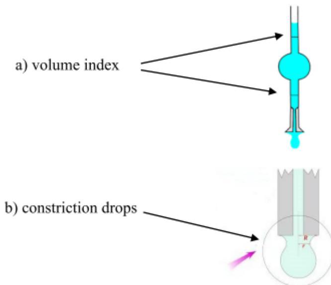
Fig.1 Stalagmometre with indicators of volume  $V$  of the bubble (a) and a drop forming at the end of the stalagmometre's capillar (b)
